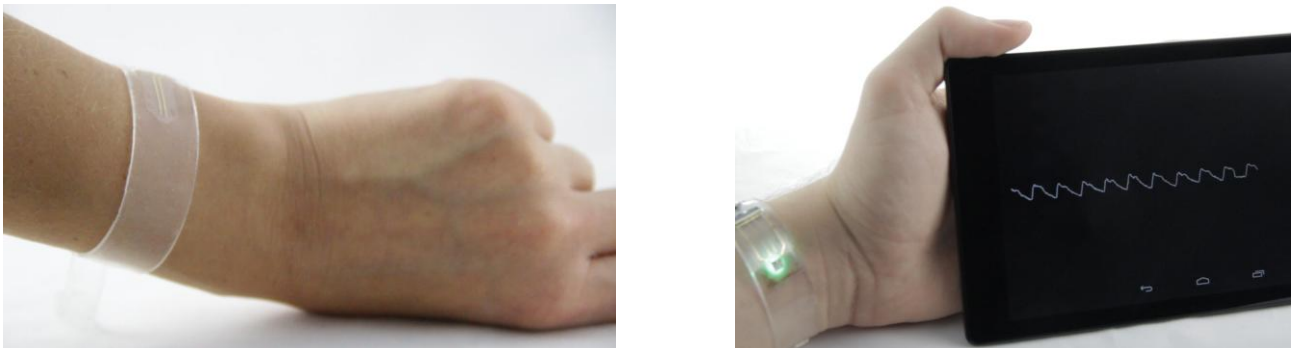
Figure 1 (a) Wrist band with graphene sensor. (B) A working prototype system in the form of a wristband, including a tablet to display the pulse in real time.
